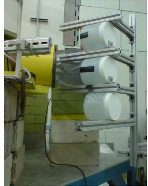
Figure 2. (a) Close-up of the beam entry onto the sample. The beam enters through the plastic pipe surrounded by lead shield blocks (green), which shield the sample and detectors from scattered radiation originating from the gamma-source. (b) Close-up of the sample-mount with three samples attached simultaneously. The sample-actuator (not visible here) is capable of moving the mount along the horizontal and vertical axes, which enables precise positioning of the gamma beam on each phantom separately. Also visible in this image is the camera used to monitor the sample-position in real-time.
