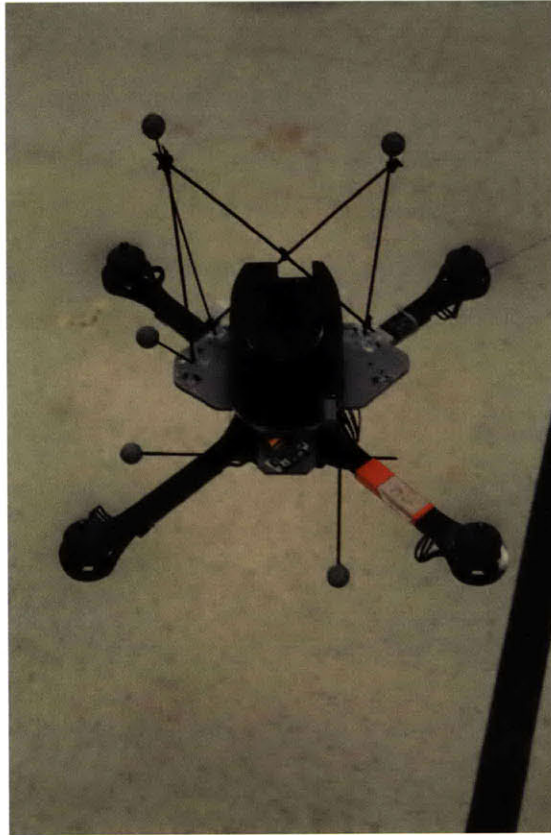
Figure B-2: Quadrotor Helicopter Equipped with Wireless Camera
