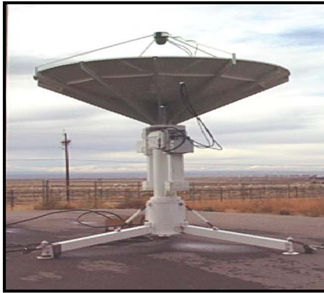
Figure 2-9. S-band Transportable Ground System Antenna
