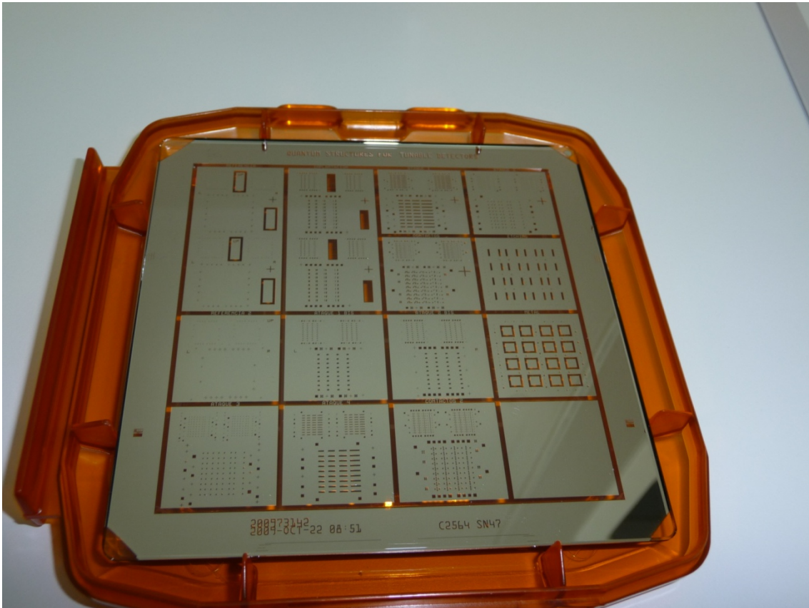
FIG. 15 Optical lithography mask manufactured for this project
