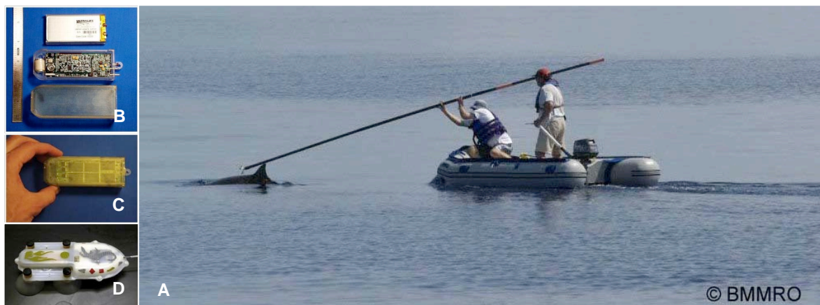
Figure 2. (A) Tagging of a Blainville's beaked whale in the TOTO, (B & C) DTAG-2 Components, (D) Complete DTAG-2 with housing and suction cups.
