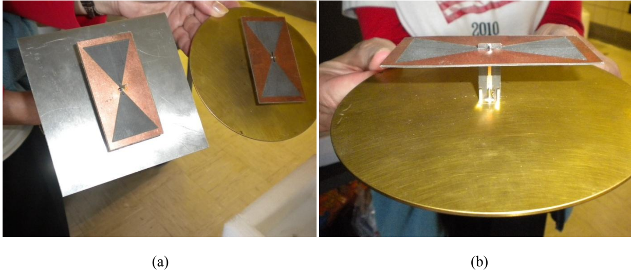
Figure 17. (a) Top view of the FTBA element over both square and circular ground planes. Only the circular ground plane was used for measurements to compare with predicted results. (b) Side view of the FTBA element showing a solder tab at the top of the feed structure soldered to a leg of the dipole.
