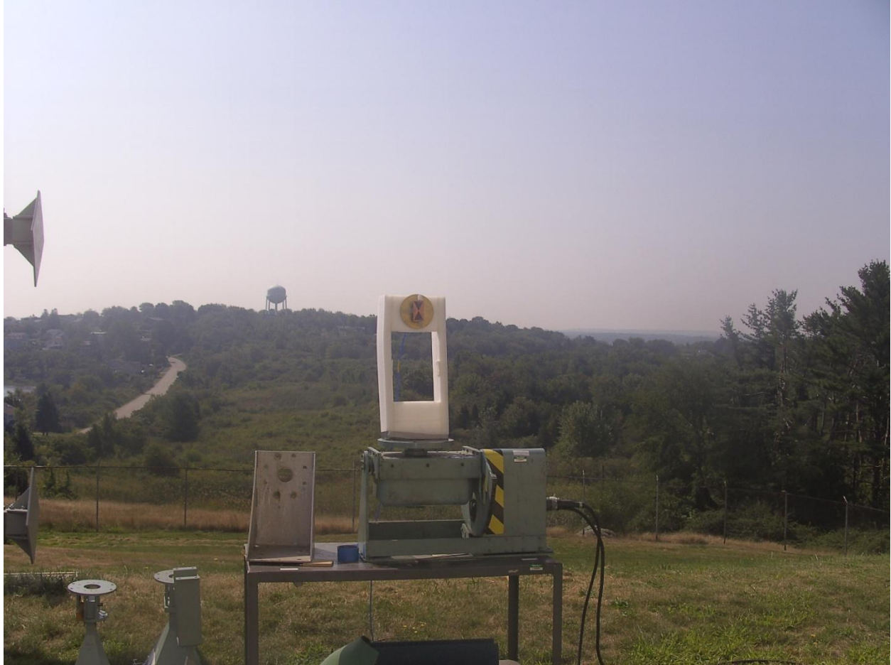
Figure 20. The FTBA on a mount at the AFRL/Ryha Ipswich Antenna Research Facility, Ipswich, MA. The standard gain horns to the left of the mount were used in the gain measurements. The white frame is foam structural support. In this configuration the antenna is horizontally polarized.
