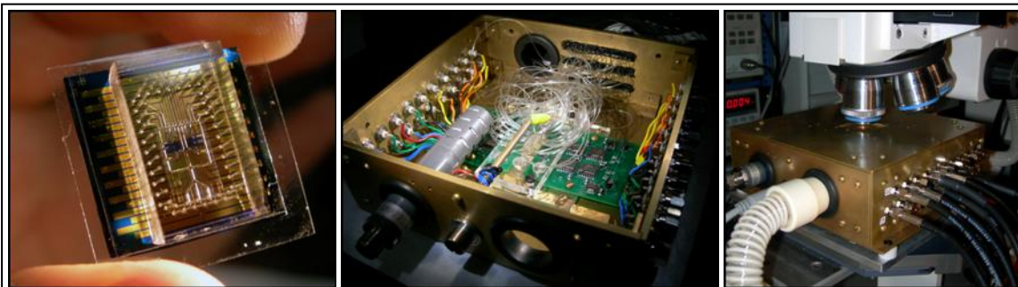
Figure 1. Left, NEMS chip encapsulated in microfluidics. The microfluidics include 40 computer operated control lines, 15 fluid input/output lines and one gas inlet line all built into an 80mm 2 footprint. The microfluidics are critical for separating the electronics from the fluids – controlling stray capacitances in particular, – enabling controlled media perfusion for long term tissue culture, controlling placement of a cell on the force sensor and precise pharmacological perturbation of the cell. Center and right, the microscope-mounted-incubator-and-sample-holder includes freedthrus for 64 microfluidic lines. 40 electrical lines. CO2 sensor. temperature
