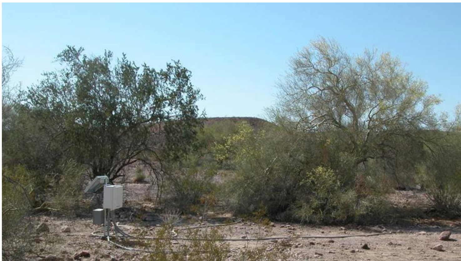
Plate 5. One of six sapflux and soil moisture stations deployed in Yuma Wash for the duration of the study.
