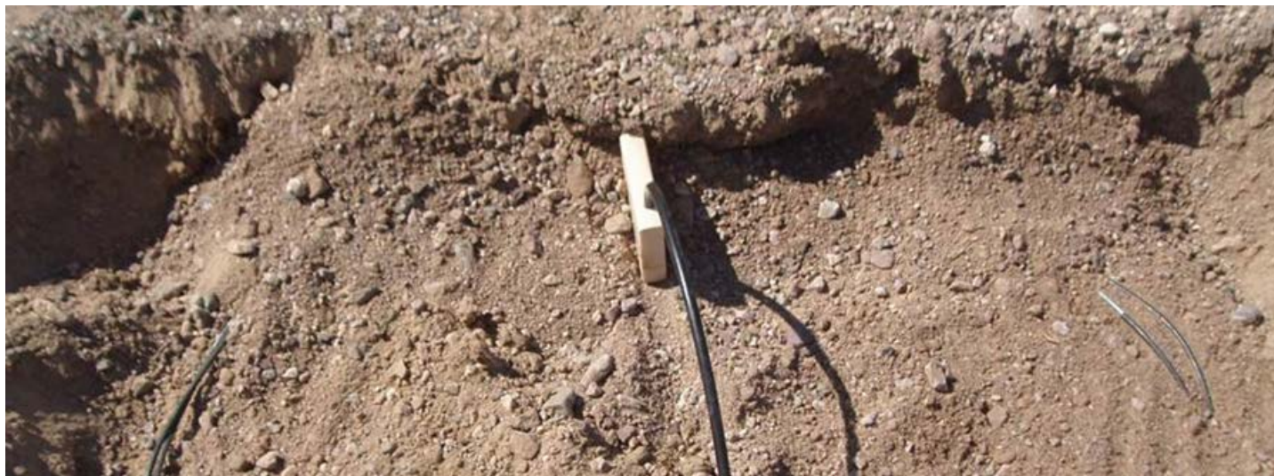
Plate 4. Soil heat flux instrumentation installed at 2.5-8cm beneath the soil surface at each of six (micro) meteorological stations in Yuma Wash. Instrumentation consisted of (1) soil water content reflectometer, (4) soil temperature sensors, and (2) soil heat flux plates.
