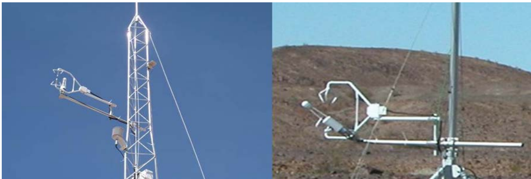
Plate 3. Sonic anemometers and gas analyzers on micrometeorological stations (ECOV1 and ECOV2) used to measure actual evapotranspiration in Yuma Wash via eddy covariance techniques.
