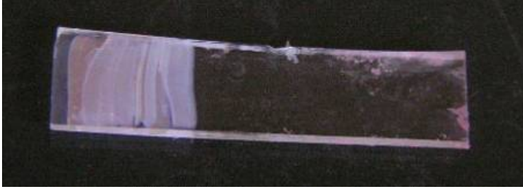
Figure 5. Image of colloidal crystal that was made using the vertical deposition method.
