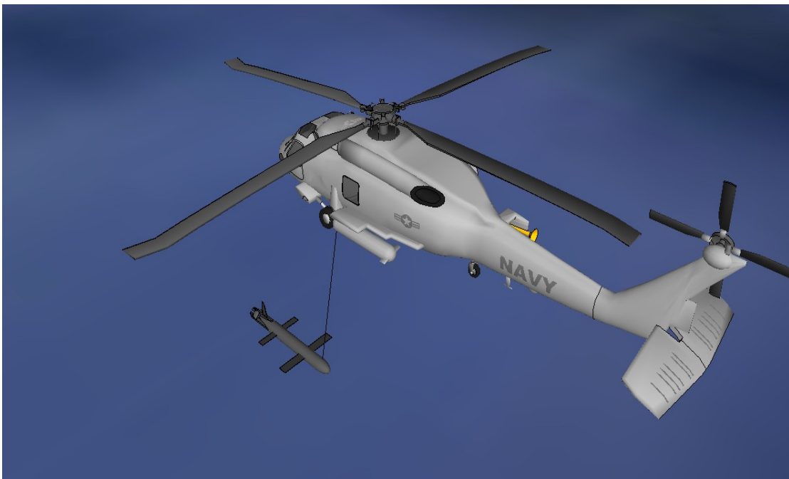
Figure 4.19: Glider Recovery Assisted by Helicopter Retrieval
