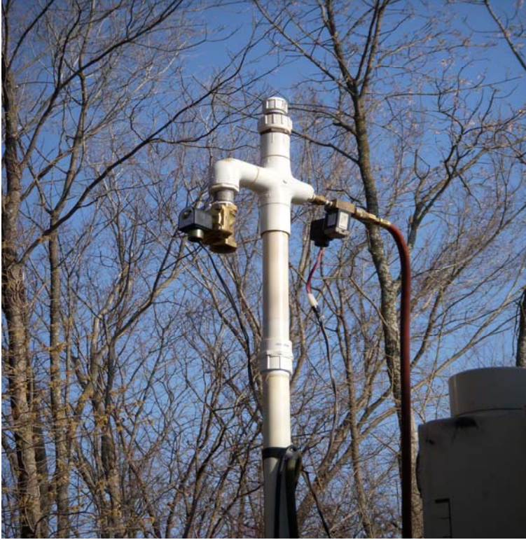
Figure 5b. Pneumatic pressure manifold with servo-controlled valves.
