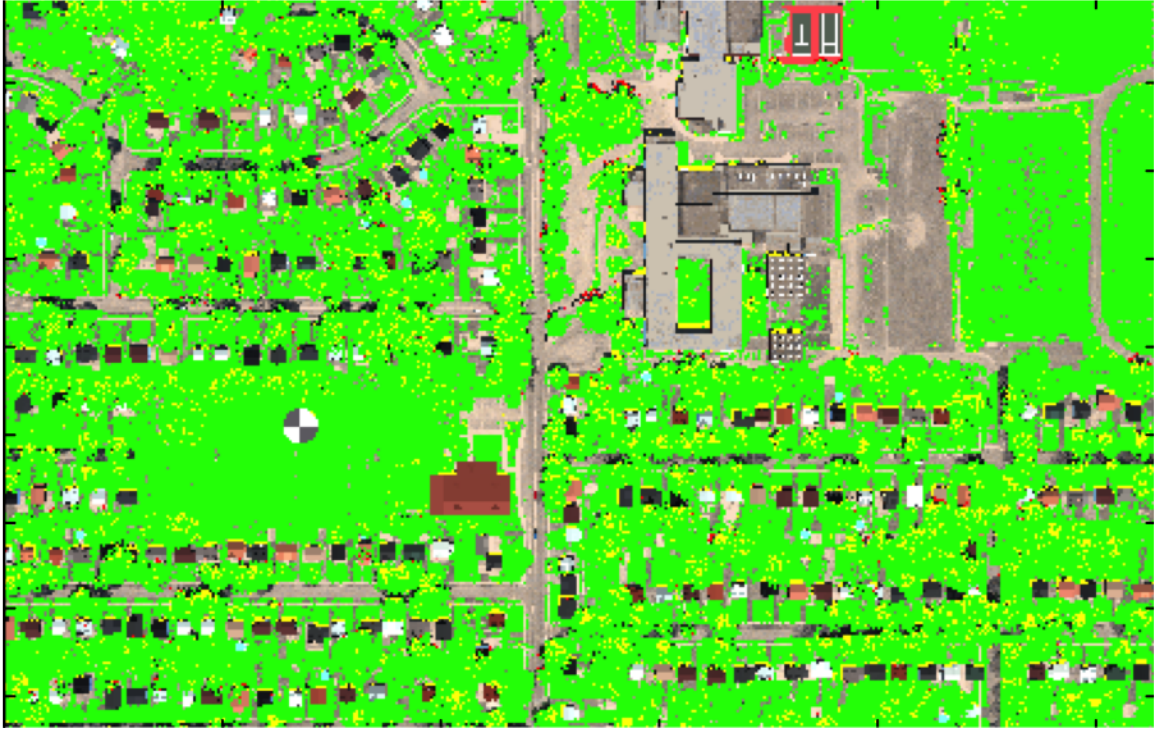
Figure 4.9: An illustration of the vegetation detection stage of background modeling. The underlying image is a pseudocolor rendering of the hyperspectral cube. The bright green and yellow colors indicate pixels which exceeded the thresholded NDVI test and were declared vegetation. According to truth, the bright green pixels are majority vegetation, and therefore represent accurate detections. The bright yellow pixels are not majority vegetation, and therefore represent false detections.
