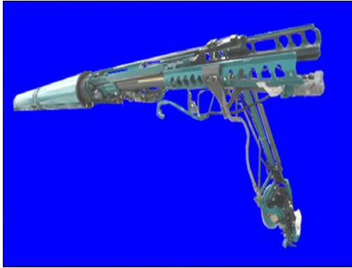
Figure 3 – AN/BLQ-11 Long-Term Mine Reconnaissance System (LMRS) (Torpedo Tube Launch and Recovery System) [White, D. P., 2007]
