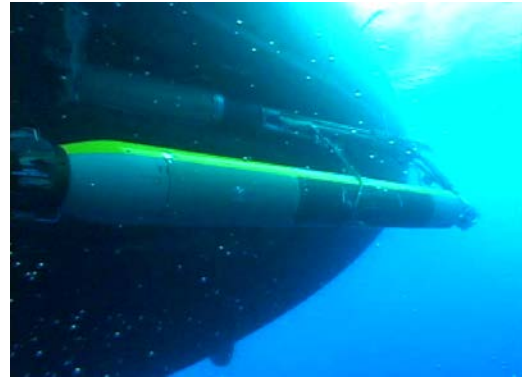
Figure 3 – AN/BLQ-11 Long-Term Mine Reconnaissance System (LMRS) (Torpedo Tube Launch and Recovery System) [White, D. P., 2007]
