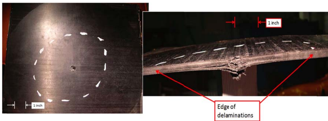
Figure 26. Post test images of the front side and cross section of the helicoidal laminate.
