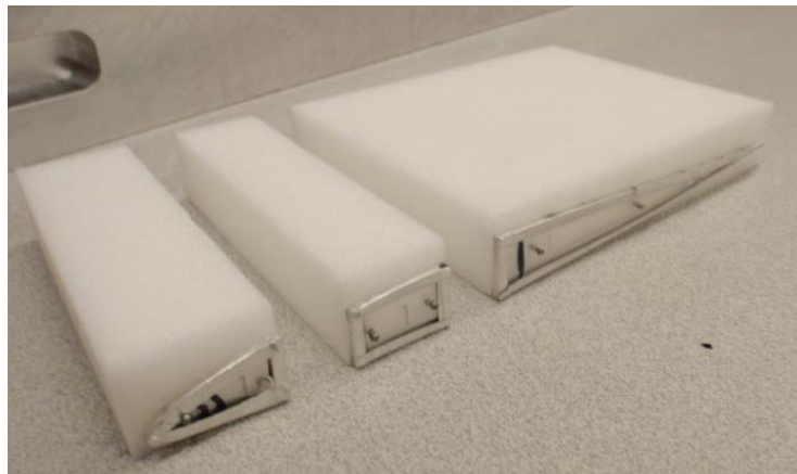
Figure 100. Uncut foam blocks with acrylic templates attached prior to sanding
