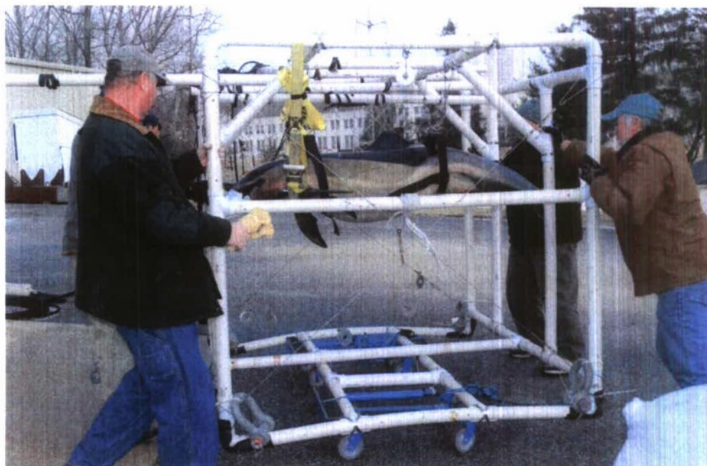
Fig. 13. The experimental subject, a 119-kg, 211-cm-long common dolphin specimen, following implantation of tourmaline sensors at the WHOI CSI Facility, suspended from a PVC-pipe frame at NSW Carderock Division on 4 February 2009. Credit: D. Ketten, S. Cramer, K. Rye, W. H. Lewis, M. Hastings.
