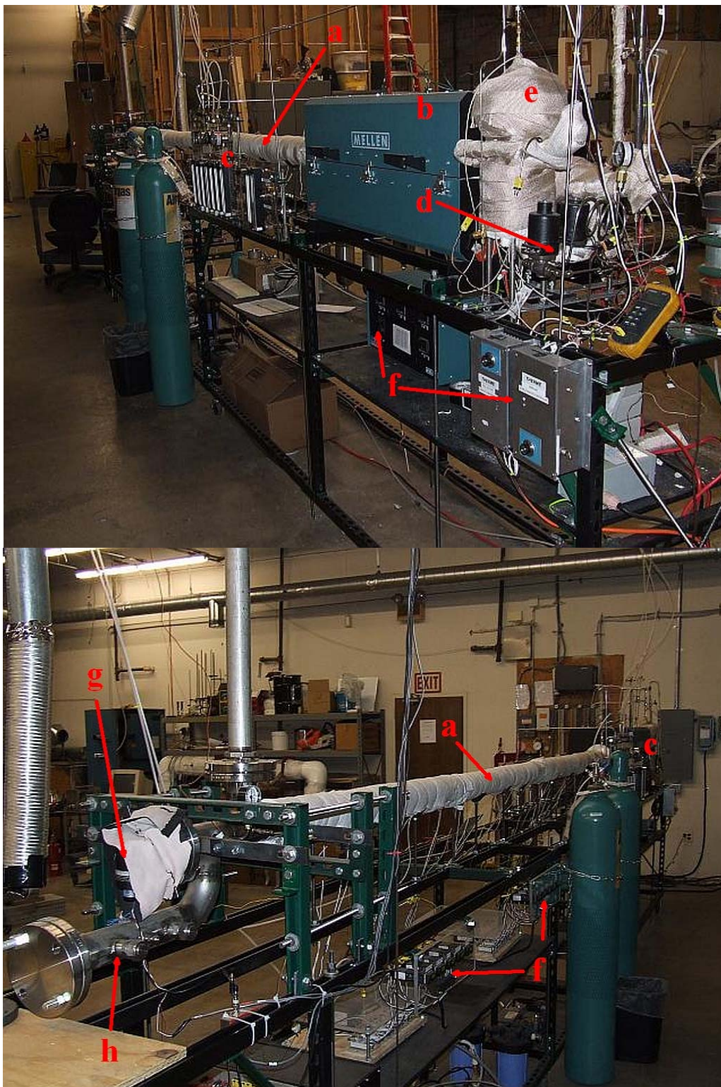
Figure 2-14: Flow reactor apparatus used for detailed phase experiments. Key: a) flow reactor tube, b) tube furnace, c) flow control panel, d) solenoid manifold, e) fuel vaporizer, f) heater controls, g) photomultiplier tube, and h) transition piece.
