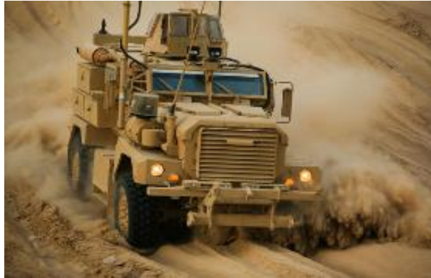
Figure 1. Cougar H 4x4 Mine Resistant Ambush Protected Vehicle on the Off-Road Course at Camp Taqaddum, Iraq
