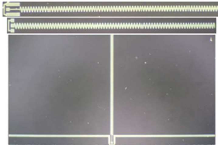
Figure 12: Fabricated antenna test structures
