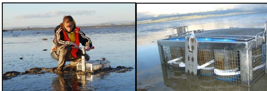
Figure 8. Pictures showing deployment of bioassay cages in the field.
