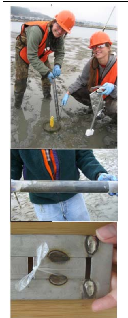
Figure 4. Pictures (top to bottom): deployment of passive sampler rods for vertical pore water profiles; sediment core; close-up of deployment rod with POM passive sampler.
