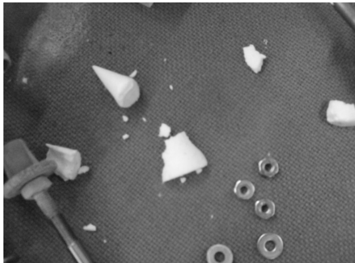
Figure 41: Early test article that failed upon removal from mold
