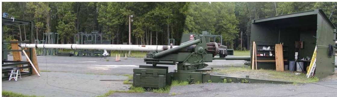
Fig. 36 A 75-mm gun used to launch projectiles at ARL
