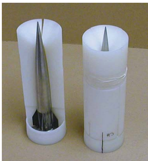
Fig. 35 Partial and complete assembly of launch package
