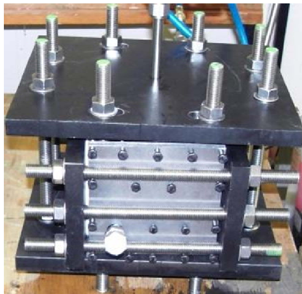
Figure 11. Generator showing Bracing Rods & Clamping Bolts
