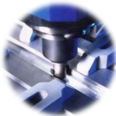
Friction Stir Welding and joining of dissimilar metals
