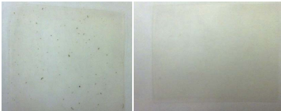
Figure 3: Membrane samples pressed between Teflon at 350 °F (left) and 270 °F (right). The brown spots that appeared are likely an indication of thermal breakdown within the material.
