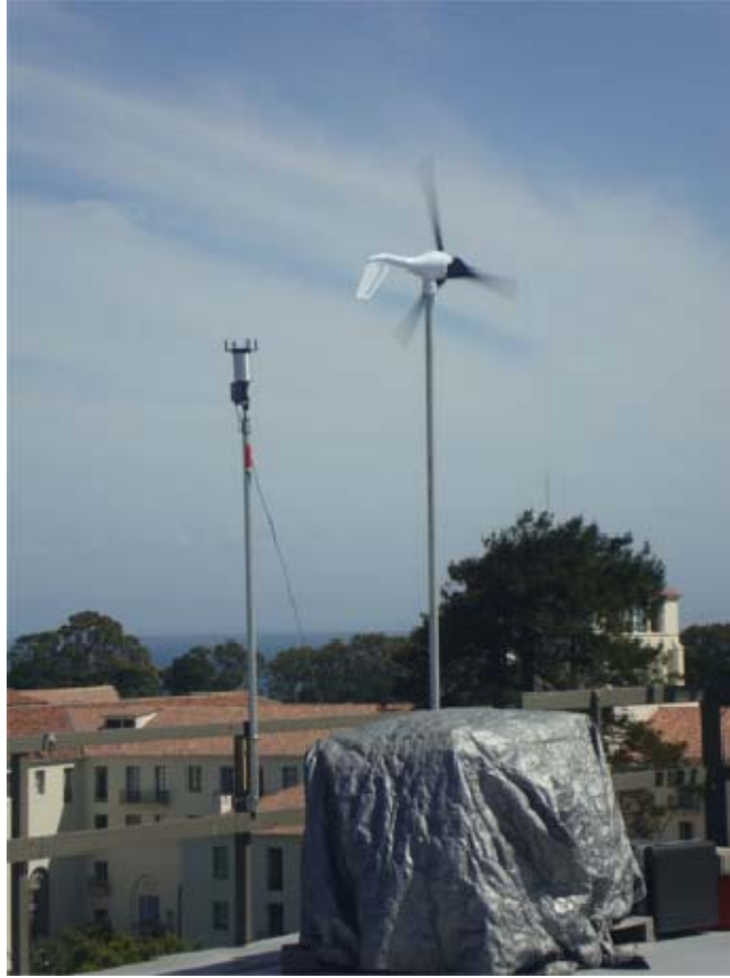
Figure 30. Photo of the Air X and Adjoining Anemometer Used in the Wind-PV Experiment
