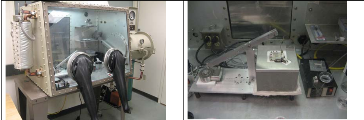
Figure 22. Glove box working environment and thermo compression bonder inside the glove chamber.
