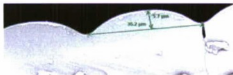
Figure 10. Cross sectional SEM image of a buckled substrate.
