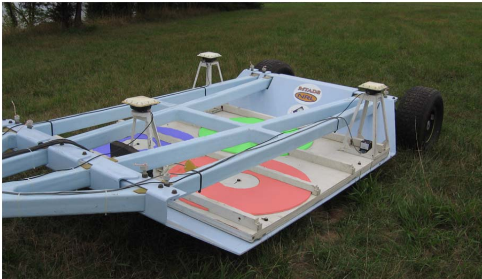
Figure 2-3 – MTADS GEM-3 array mounted on the EM sensor trailer. In addition to the three GEM-3 sensors, note the three GPS antennae and the IMU for platform motion measurement. The sensors are false-colored as discussed in the text. The IMU is the small black box mounted under the MB2 GPS antenna.
