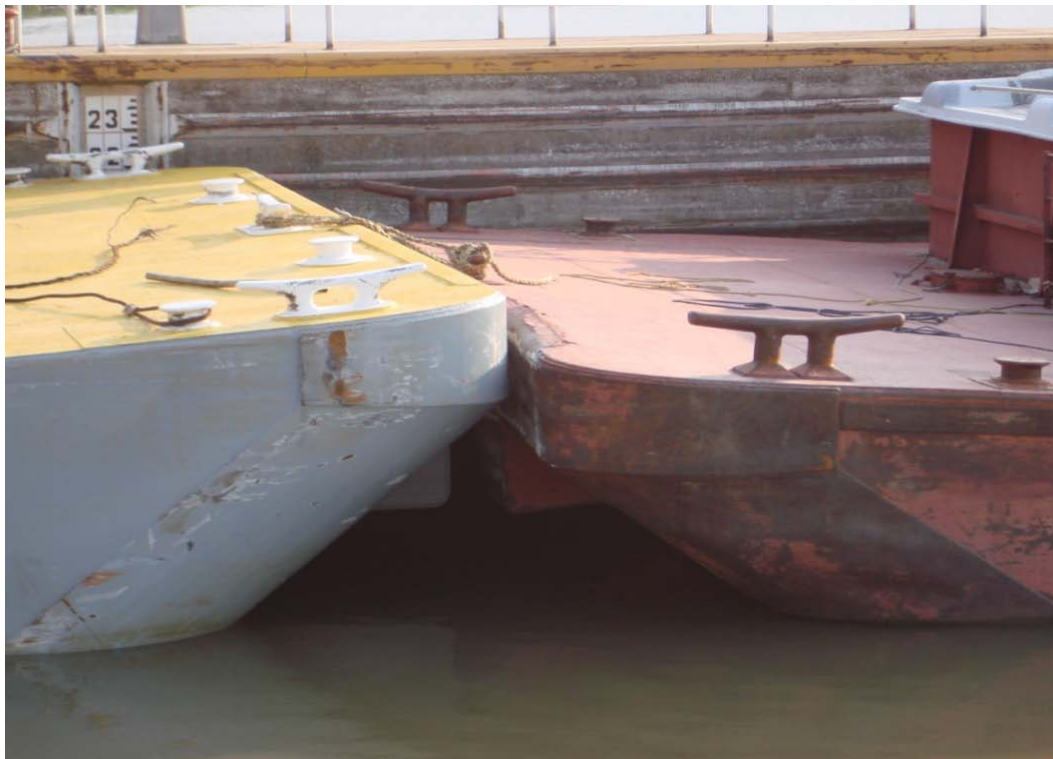
Figure 2.20. View of damage to barges that hit the guide wall at Newt Graham Lock and Dam 18.
