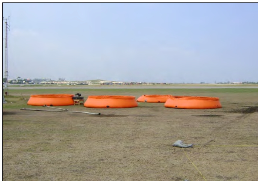
Figure 18. Four 2500-gal Capacity Onion Bladders Stored Water for Later Use
