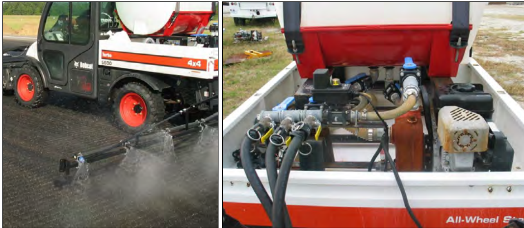
Figure 5. The Folding Spray Bar System Includes a Pump and Water Tank
