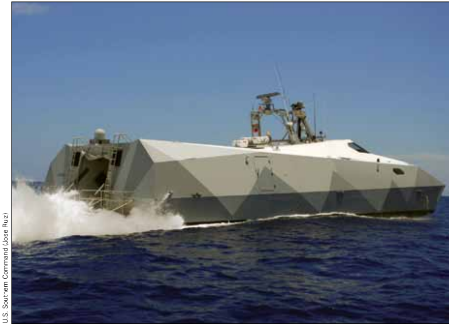
Experimental vessel Stiletto , manned by a crew of Army and Navy mariners and U.S. Coast Guard Law Enforcement Officers, trains for counter-illicit trafficking deployment to the Caribbean. An example of innovative design and construction, the Stiletto is lightweight, able to operate in shallow waters, easy to maintain, and fast (up to 50 knots in calm seas).
