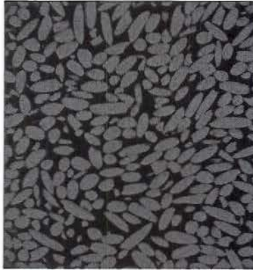
Figure 2.7. A cross-section of the voxel pack after smoothing. Notice that the particles have a constant density throughout in contrast to the variation seen in Figure 2.5(b).
