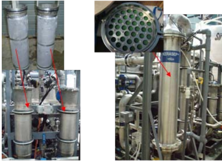
Figure 8. Photos of Tubular Filter Skid (left) and Membrane Filter Skid (right)
