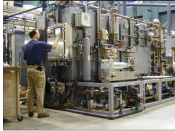
Figure 12. Photos of NSWCCD Non-Oily Wastewater Laboratory Setup for Pilot and Full-Scale Tests
