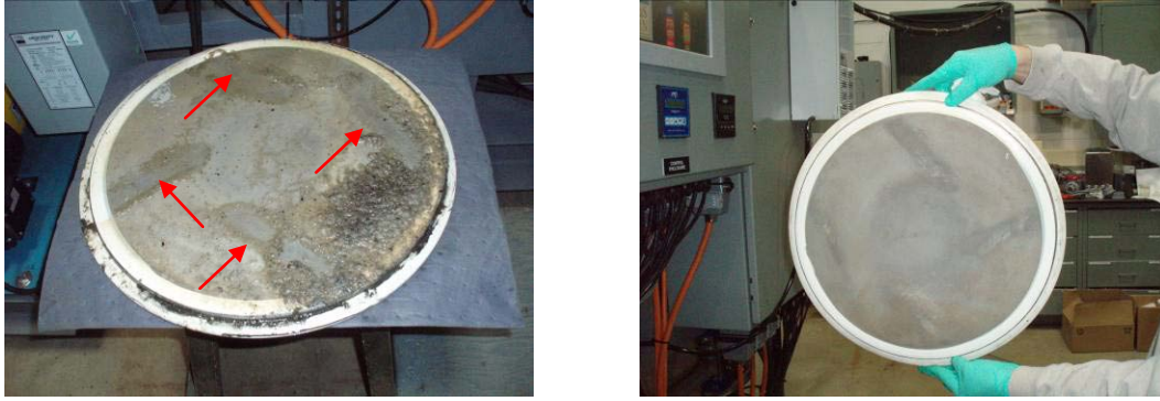
Figure 14: Photos of the Clogged 200-mesh screen (left) and the Cleaned 200-mesh screen (right)
