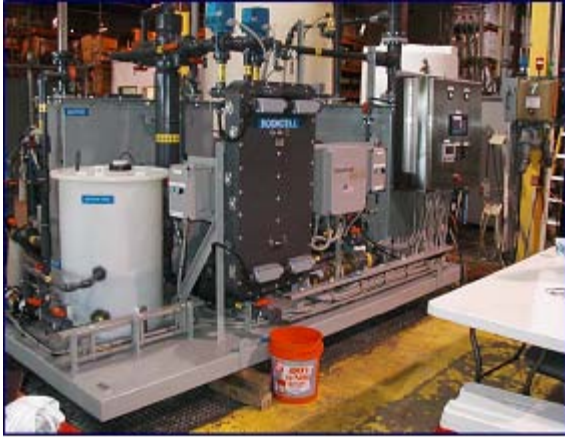
Figure 12. Photos of NSWCCD Non-Oily Wastewater Laboratory Setup for Pilot and Full-Scale Tests
