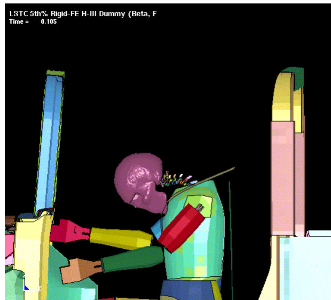
Figure 19. Frontal collision simulation using the NAVAIR high fidelity cervical spine and head model
