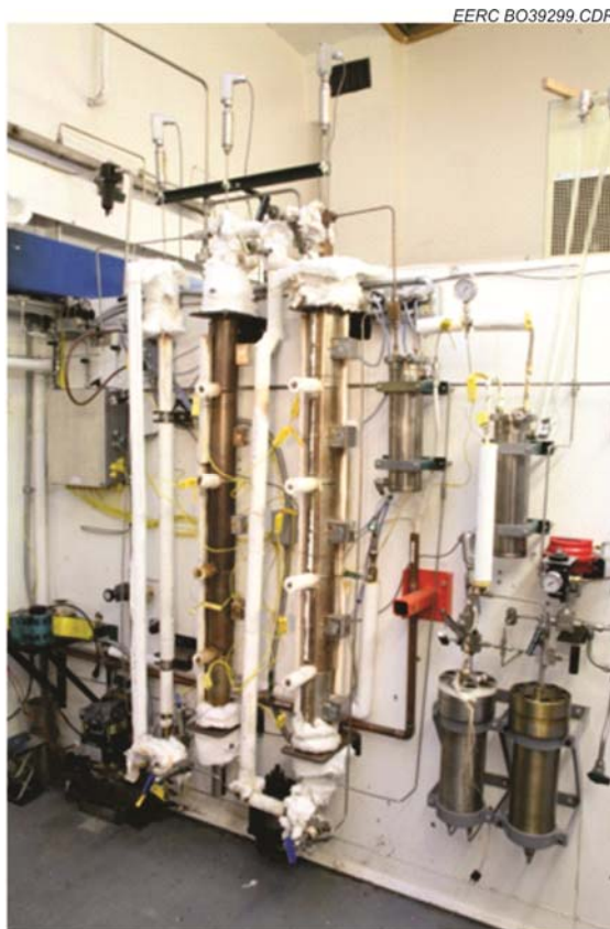
Figure 2. Reactor system used to convert algae oil to JP-8.
