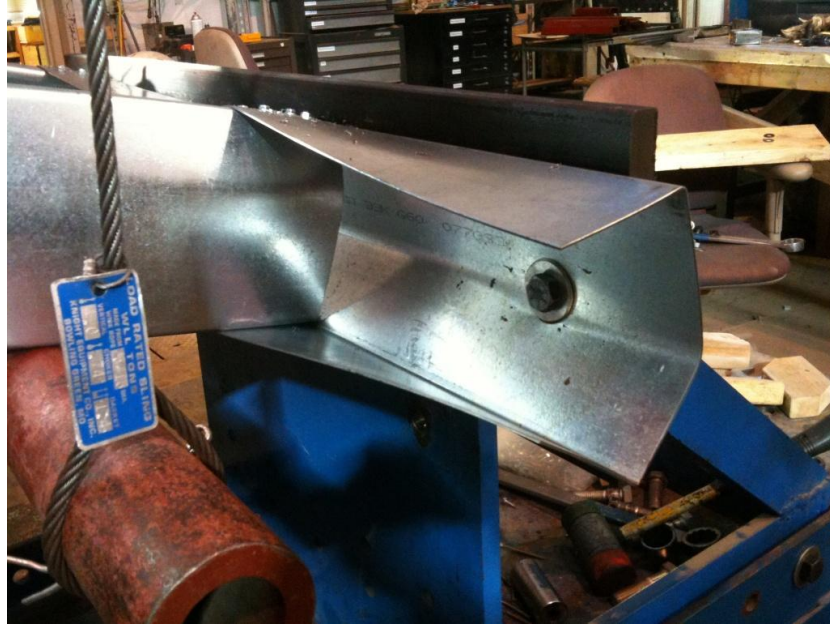
Figure B-1. Full-Length Sample 18 after Failure
