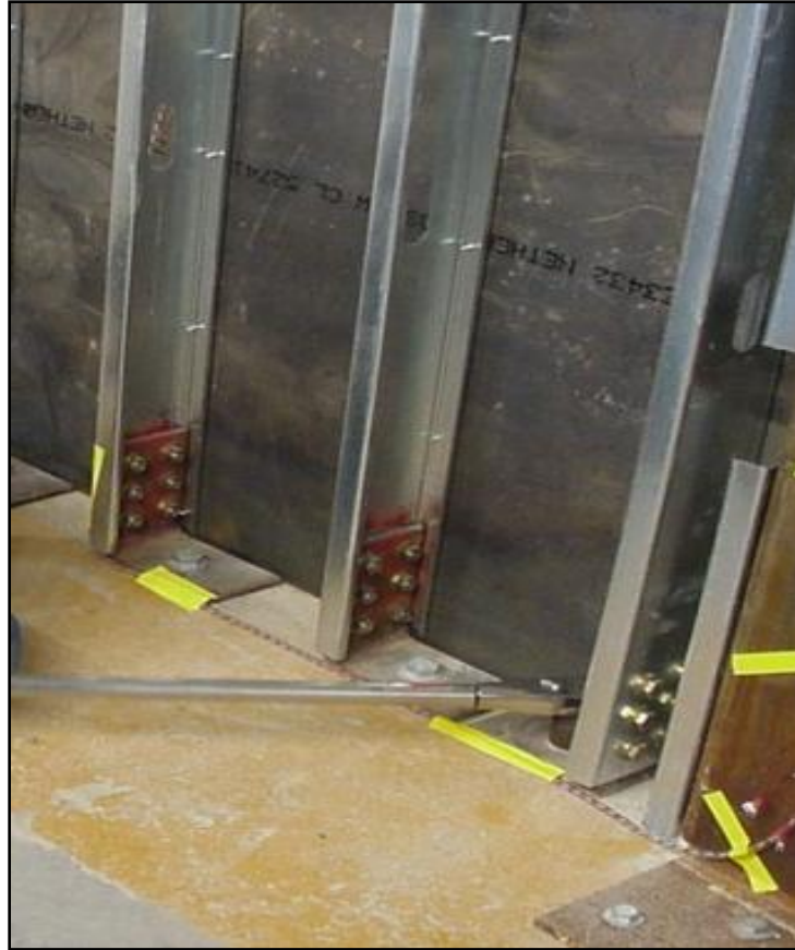
Figure 6. BREW Steel Stud Connection Detail [10]
