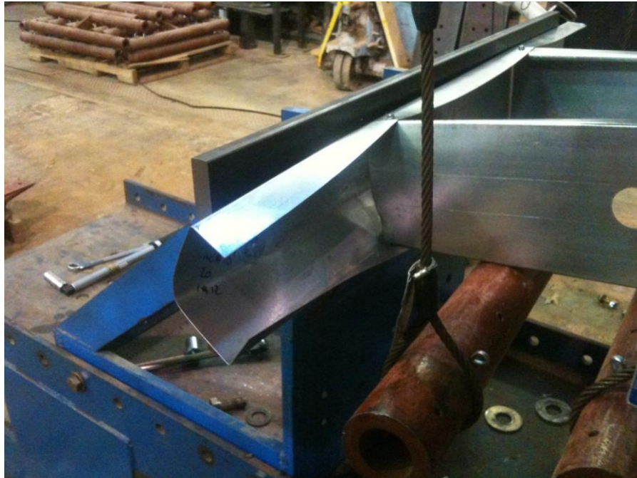
Figure B-9. Full-Length Sample 20 after Failure
