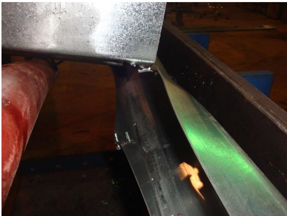
Figure B-36. Full-Length Sample 52 after Failure
