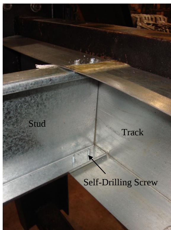
Figure 16. Typical Connection Detail
