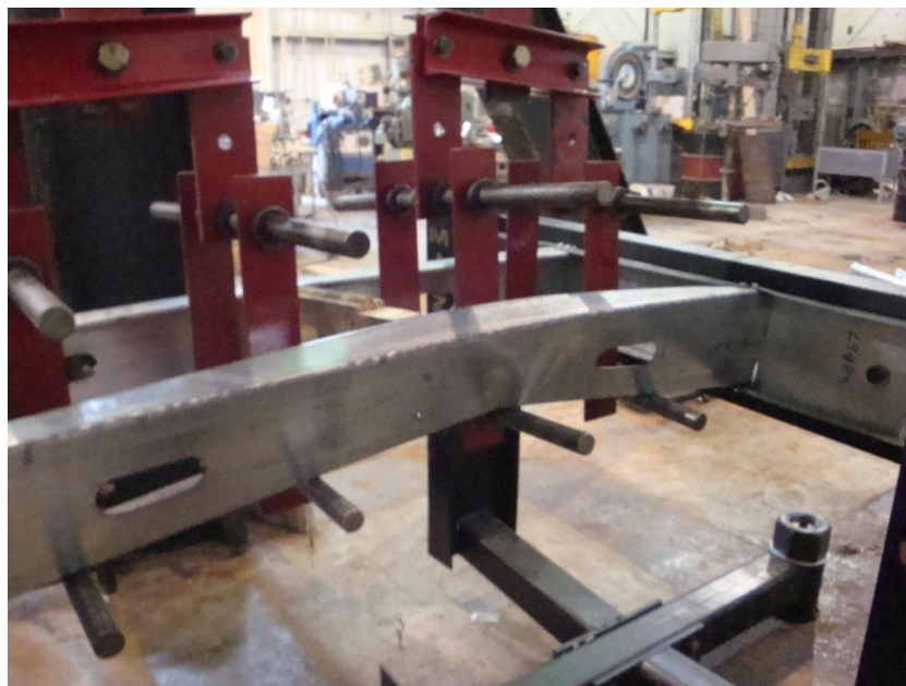
Figure 33. Stud Crippling at Mid-Span
