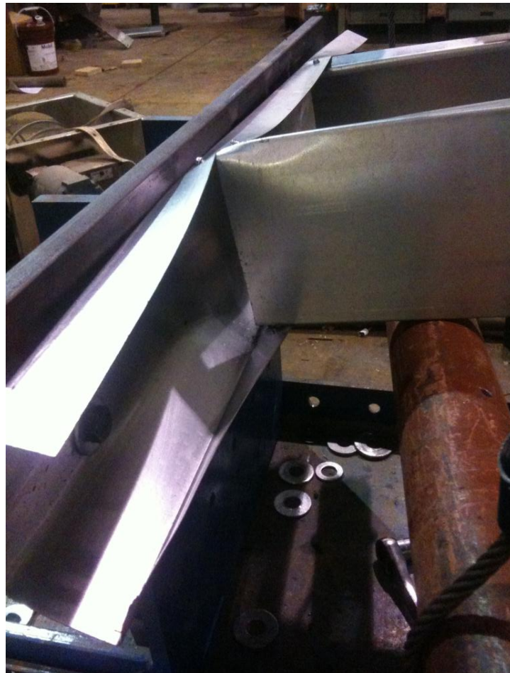
Figure B-2. Full-Length Sample 18 after Failure
