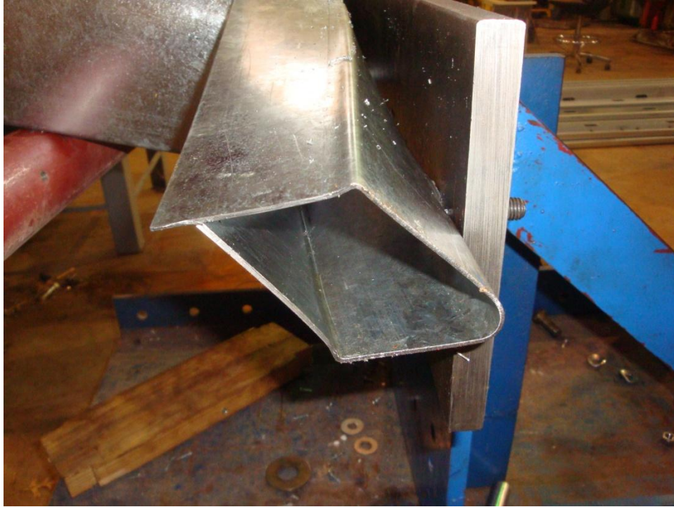
Figure B-15. Full-Length Sample 36 after Failure
