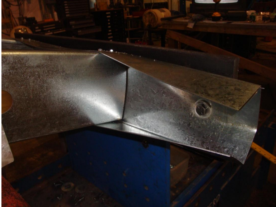
Figure B-21. Full-Length Sample 43 after Failure
