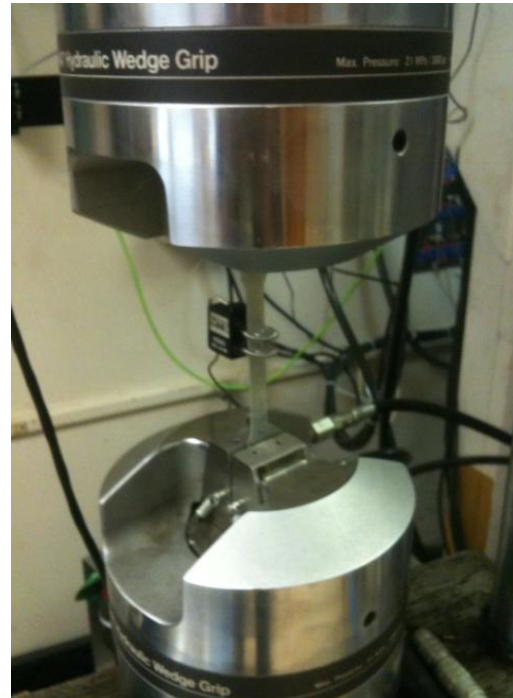
Figure 18. Coupon Testing MTS Set-up
