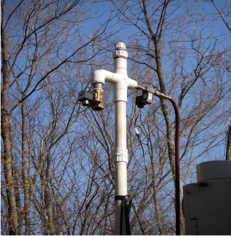
Figure 5b. Pneumatic pressure manifold with servo-controlled valves.
