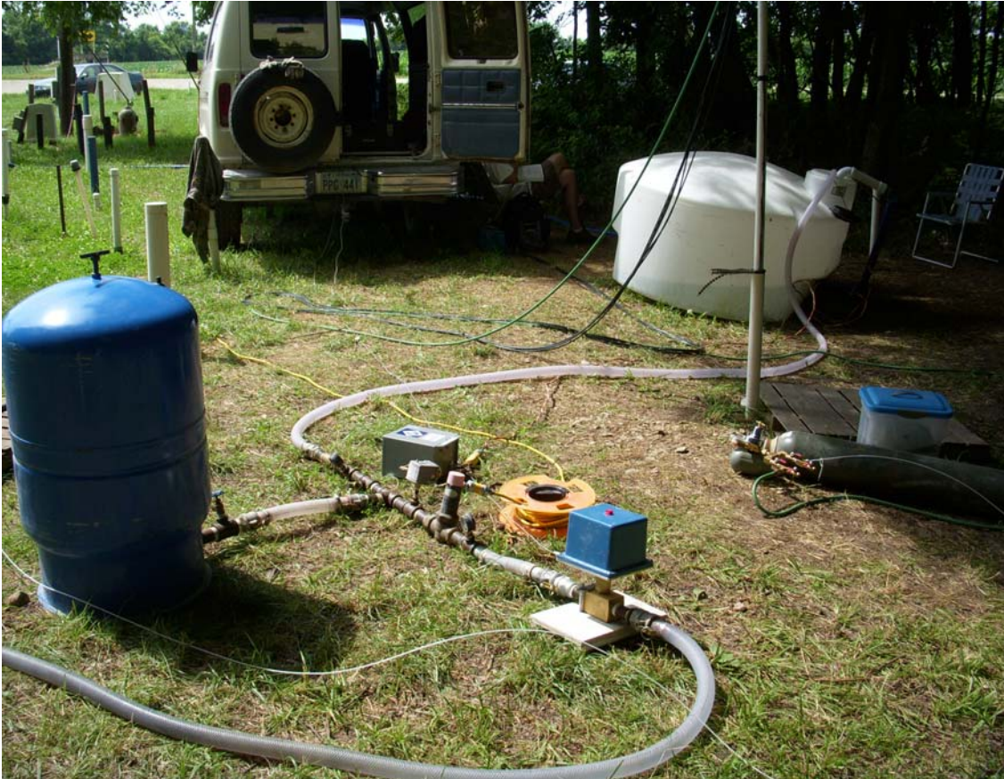
Figure 5c. Pumped hydraulic injection apparatus for the CPT.
