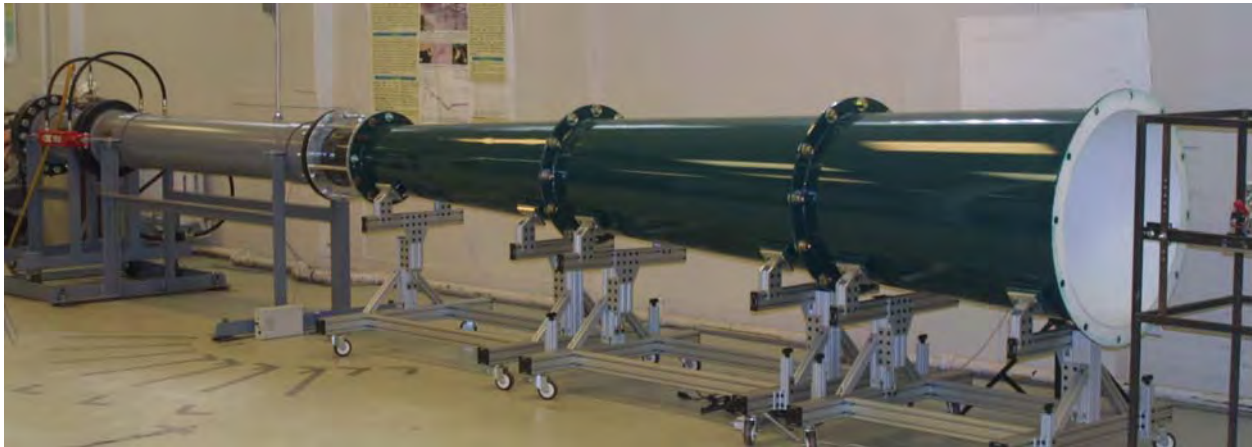
Figure 1: Wayne State University shock wave generator. This shock tube is housed at the Bioengineering Center. It is approximately 26 feet long and 30 inches in diameter at the open end. At the opposite end is the driver, which is 30 inches long and 12 inches in diameter.
