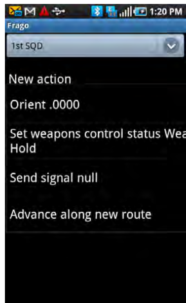
Figure 16: List of possible fragmentary orders that can be given to a unit via the Android Smartphone interface.
