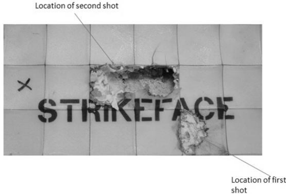
Figure 1: Ceramic Armor after Ballistic Testing
