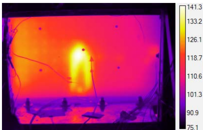
Figure 147. Temperature distribution on the test article for the +50 °F case
