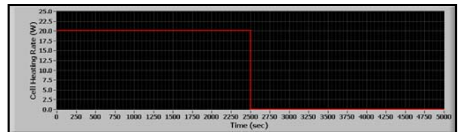
Figure 14: Step-Change Cell Heating Rate
