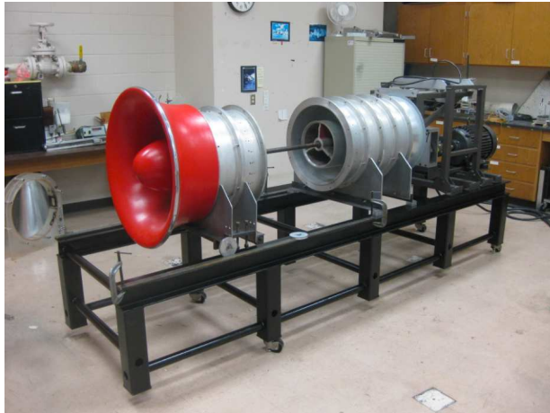
Figure 2.1: TAMU 1.5 stage low speed axial flow compressor.
