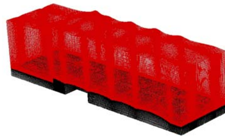
Figure Ost-3: Domain configuration for fluid-thermal validation simulation.
