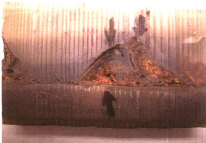
Figure 4. Cross section of tubercle and cast iron pipe from DWDS.
