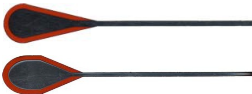
Figure 2. New generation platinum (top) and aluminum (bottom) sensor electrodes.
