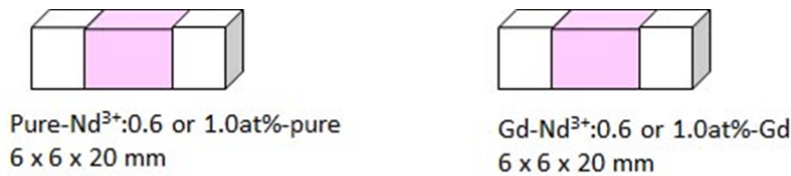
Fig.1 Three layer composite ceramic slabs used in this measurement.
