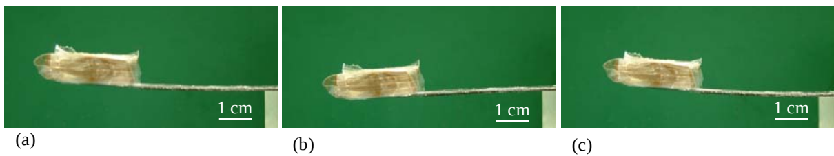
Figure 4 Deflection of PVC-CFRP laminate in thermal cycling under a load (28g of coins) (a) at 300 K before heating (b) at 340 K (c) at 300 K after cooling
