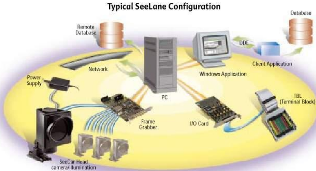
Figure 13. Typical 2-Lane LPR Configuration
